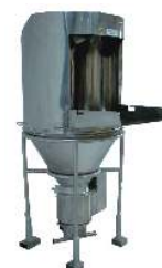
FlexiSieve incorporated into Sack Tipping Station.
