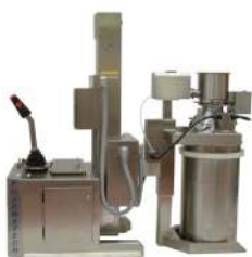
Mounted on mobile hoist for safety sieving from drum into process.
