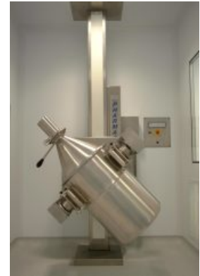
Hoist Blender with a 200L drum & cone
