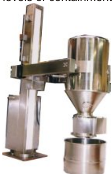
Drum Hoist with a 200L drum
