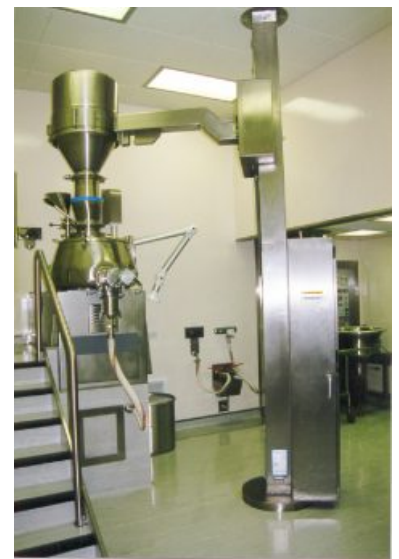
Drum discharging into a Diosna Mixer Granulator
