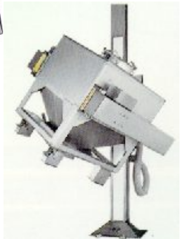
Hoist Blender with 'C' Frame Arms blending a 1500L IBC
