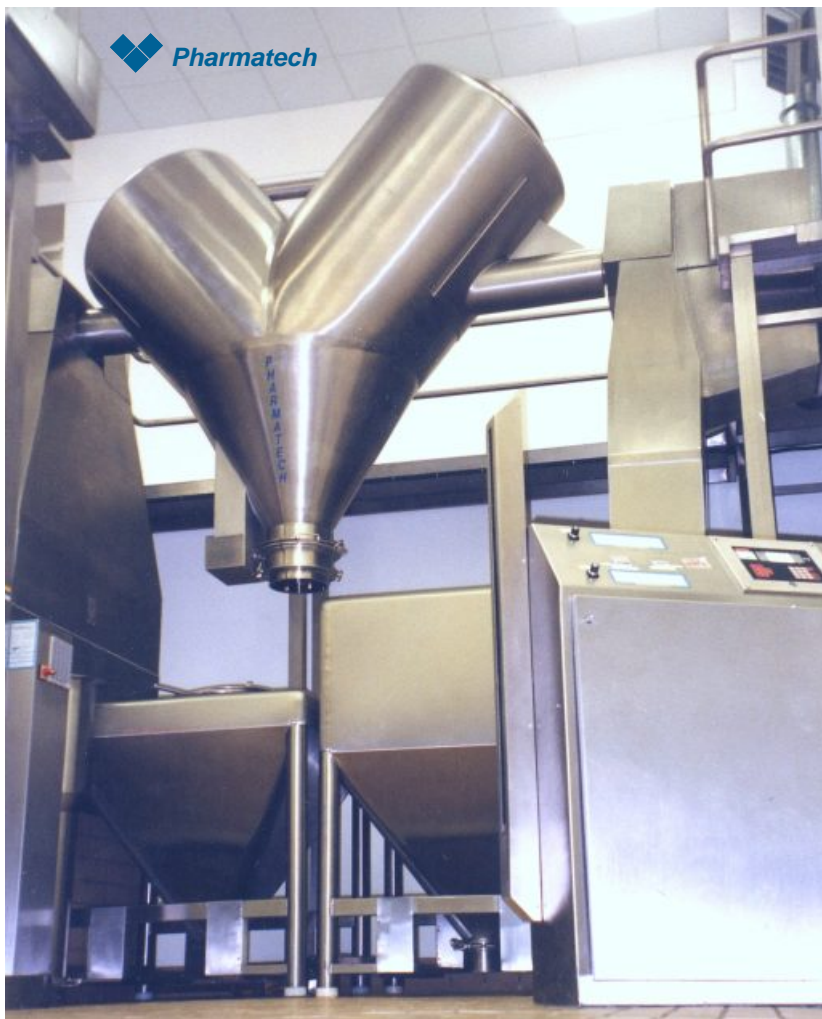
3500 litre V-Shell Blender, double plinth design The blender is loaded directly from IBCs presented on a hoist
