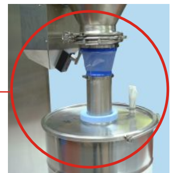
A V-Shell Blender is discharged into a drum using a flexible dust tight connection
